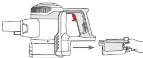
2. Slide the new battery into the motor compartment. Push until it locks into the motor compartment.
