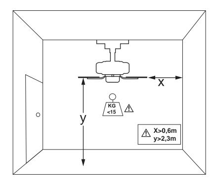
The distance between the fan blades and the wall should be at least 0.6m.
